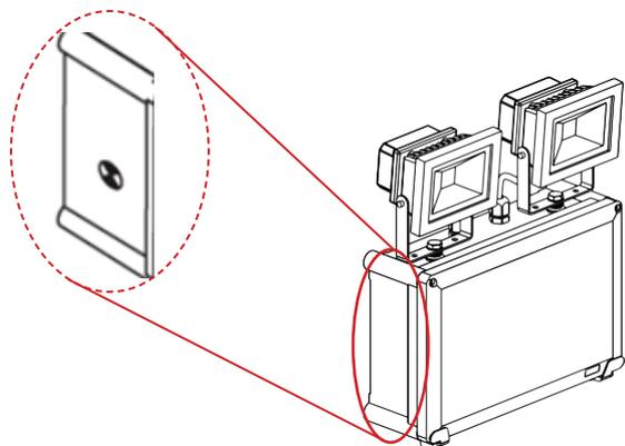
The test switch on this product is a magnetic type so that the weatherproof seal does not have to be opened. To perform a manual test, hold a magnet against the product surface near the **"Magnetic Test Switch"** label.
