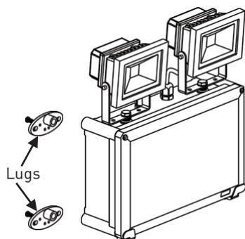
1. Fix the box to the wall either directly through the 4 channels in the box or using the lugs. Use 8 to 12 gauge screws (not supplied).
